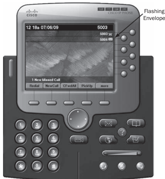
FIGURE 8.1 Flashing envelope MWI
